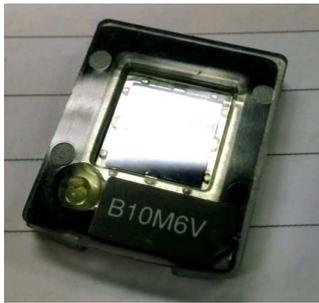
Fig. 2: Digital PCR chip
